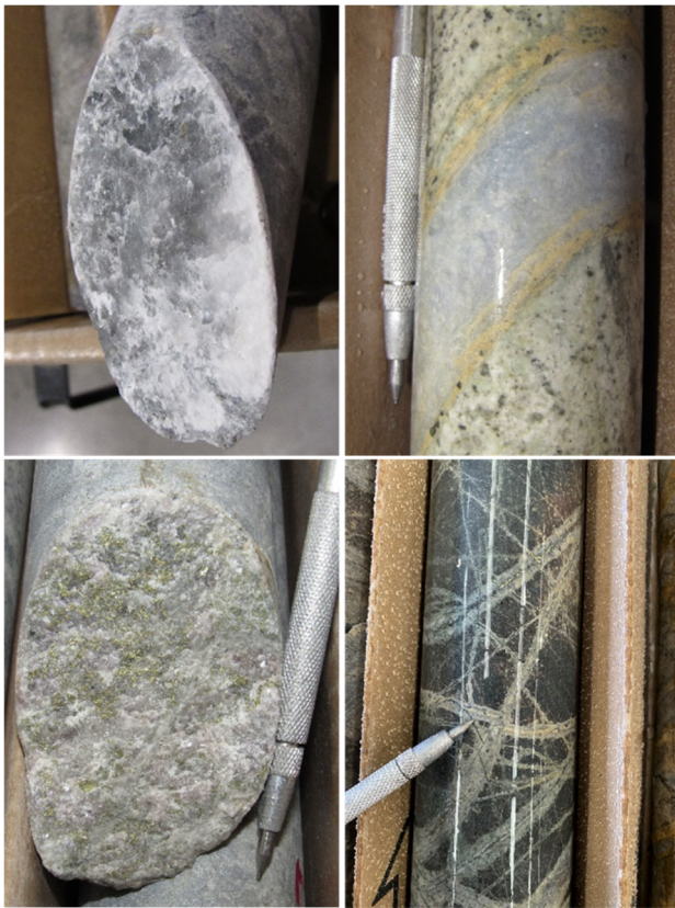
Figure 3 Examples of open and cemented veins in drill cores.
