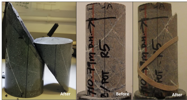
Figure 6 UCS-TCS test influenced by veins, forming a discrete (left) and combined (right) failure mode.
