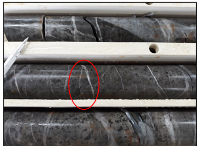
Figure 3 Calcite & Gypsum veins captured during discontinuity and defect logging.
