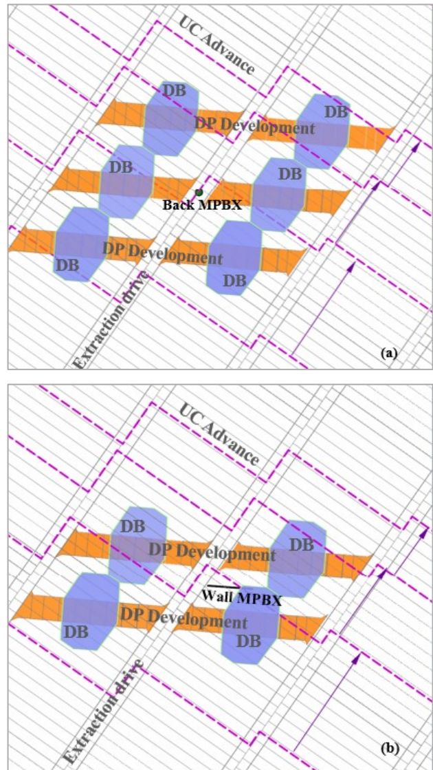
Figure 5 MPBX positions, back (a) and wall (b), with respect to undercutting (UC face advance, drawpoint (DP) drives development, and drawbell (DB) opening) stages.
