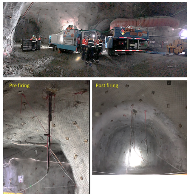
Figure 8 Preconditioning by blasting full-field trials PMCHS (QMR Blasting 2019).
