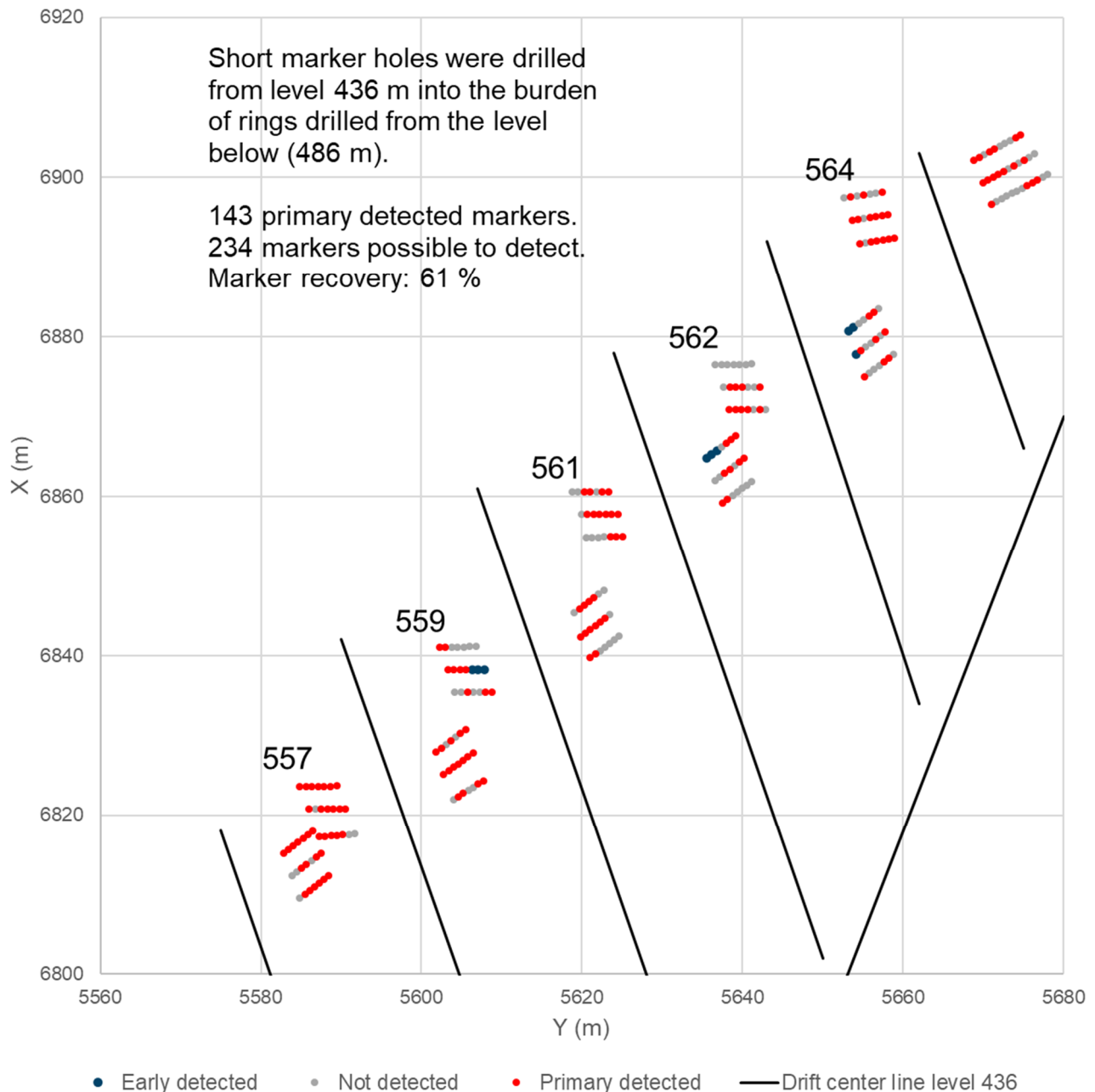
Figure 8 Top view of markers installed in short holes at level 436 and primary detected at level 486. Planned drifts center lines at level 436 are shown in black. The numbers 557-564 represents crosscuts at level 486.
