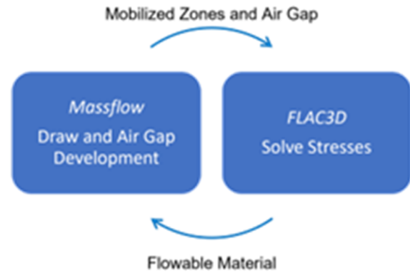
Figure 2 Conceptual scheme of the hybrid FLAC3D-MassFlow approach (after Fuenzalida et al., 2018).
