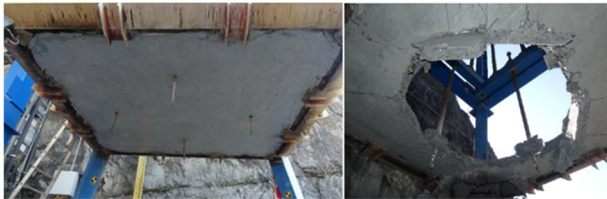
Figure 12 Ground Support System S-A1: Pre and Post Impact Test Configuration.
