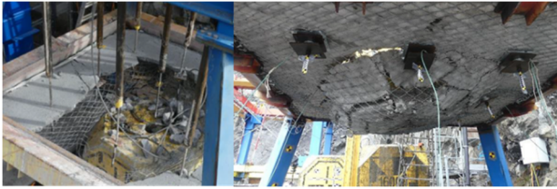
Figure 5 Examples of Ground Support System Post-Drop Test: Heavy Damage and Breach (Left), Successful Retention of Falling Mass (Right).
