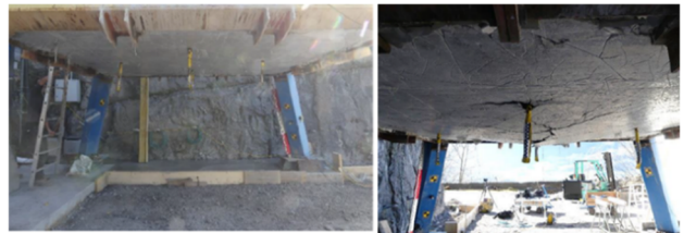
Figure 14 Ground Support System S-A2: Pre and Post Impact Test Configuration.
