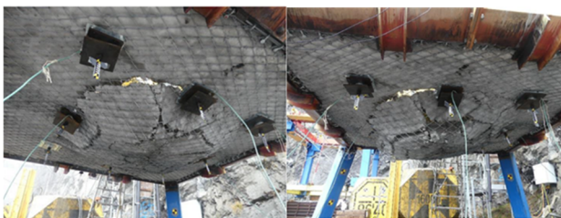
Figure 16 Ground Support System S-A2: Pre and Post Impact Test Configuration.
