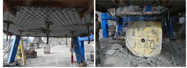
Figure 19 Ground Support System S-B1: Pre and Post Impact Test Configuration.
