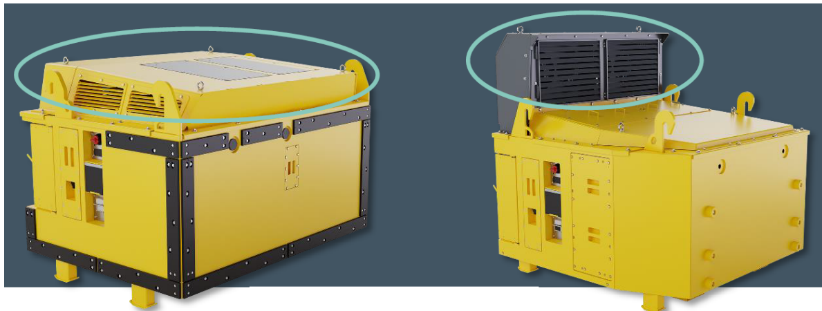
Figure 3 The extent of the thermal management system of the battery of ST14 LHD (left) and MT42 truck (right) (courtesy of Epiroc).
