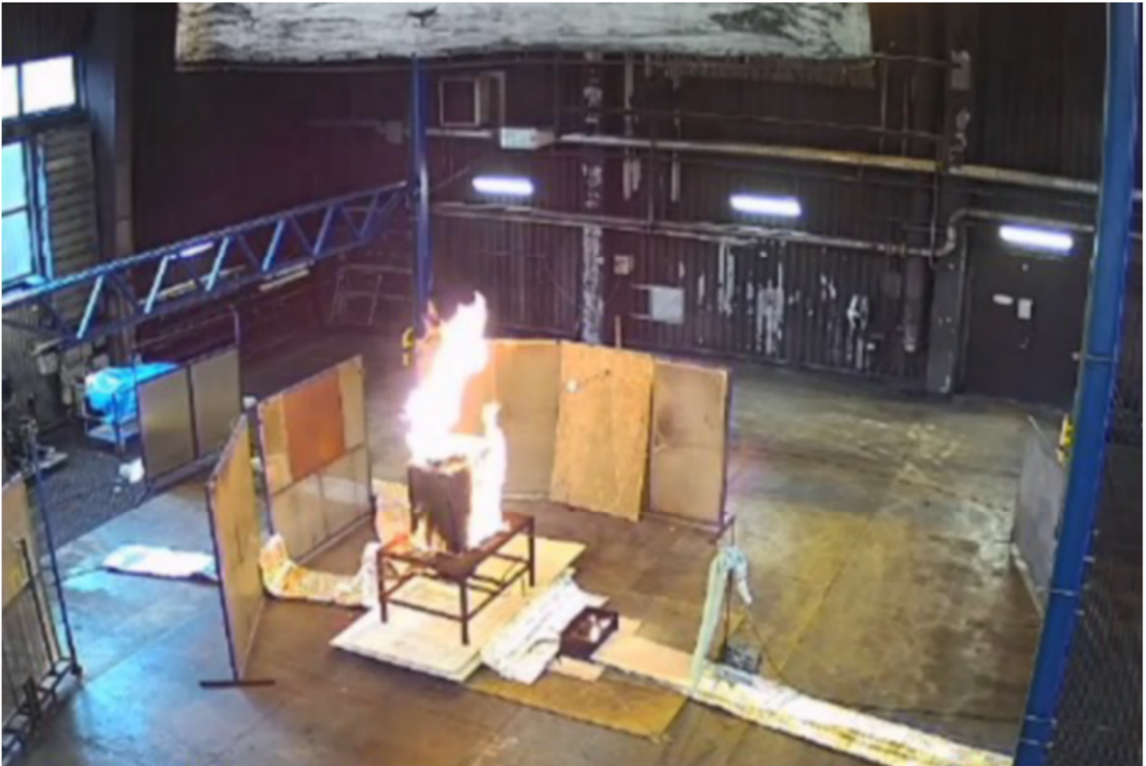
Figure 1 Full-scale fire test on Epiroc's battery sub-packs (Willstrand, 2021).
