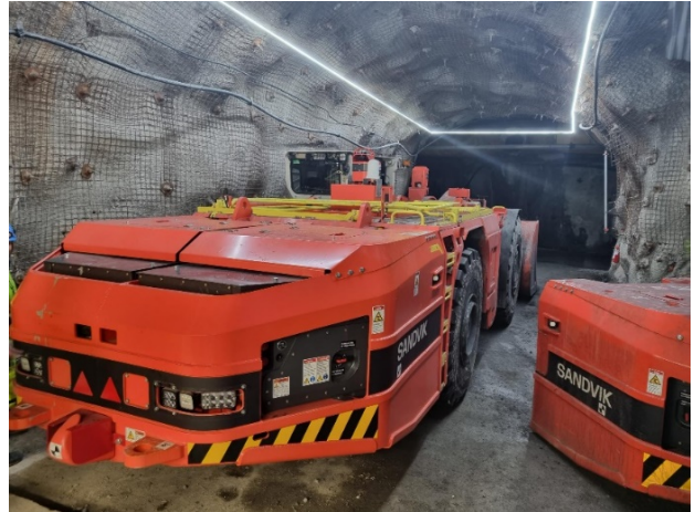
Figure 9 LH518 in the charging bay.
