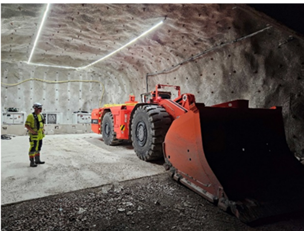
Figure 6 Worker next to LH518iB in the underground charge bay.
