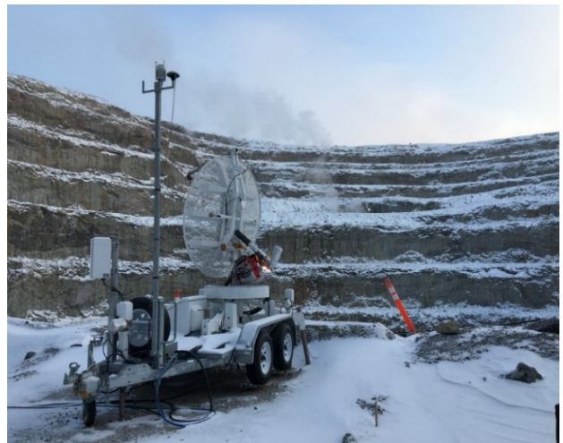
Figure 14 Radar monitoring system at the Diavik Mine.
