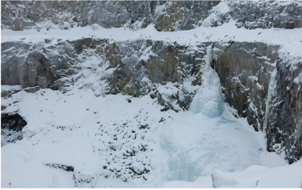
Figure 11 Snow and ice accumulation in the muckpile of A418 SLR stope.
