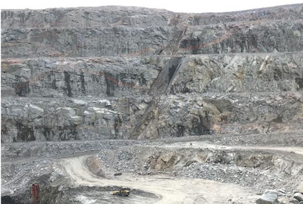
Figure 17 Stubley's fault exposed in A21 pit.
