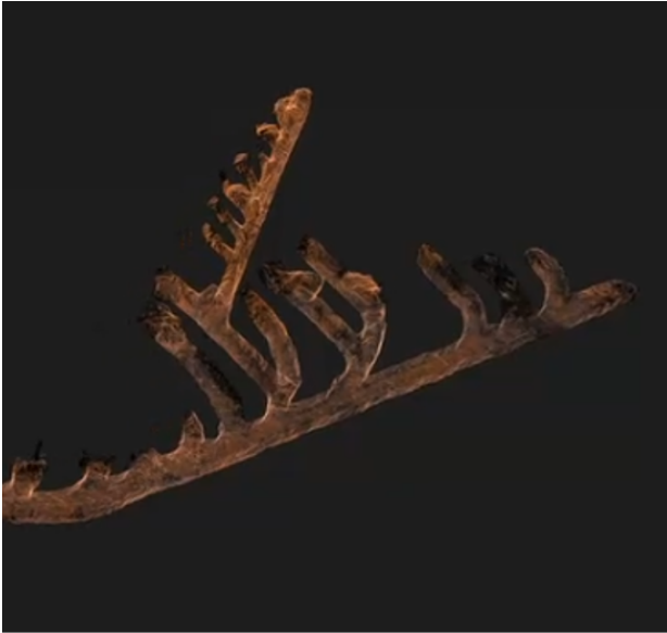
Figure 6 Laser scanning of accessible areas in Block 2 including foot wall raise.
