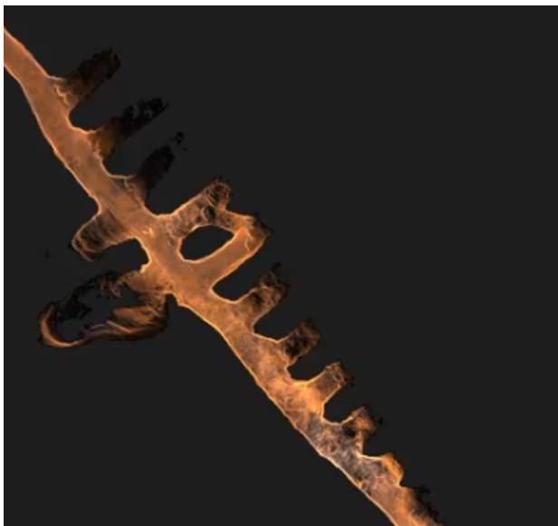
Figure 10 Laser scanning of accessible areas in Block 3, including one connection between extraction- and blasted drift.
