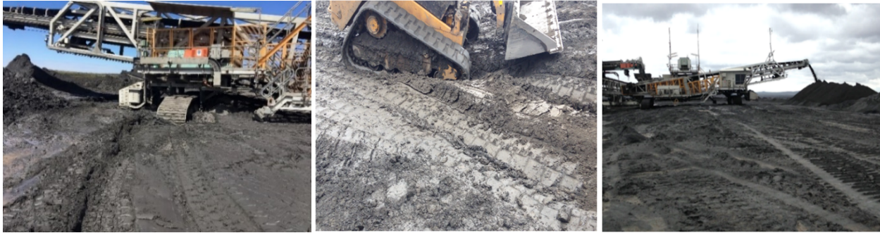
Figure 10 Mechanical stacking equipment operating in upset condition – high moisture tailings
