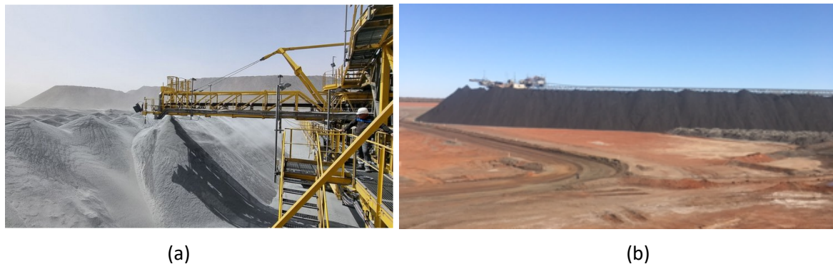
Figure 9 Mechanical stacking methods. (a) Filtered tailings stacking by retreating method; (b) Filtered tailings stacking by radial advancing method
