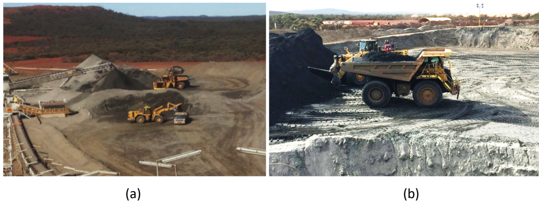
Figure 11 Emergency storage and handling. (a) Emergency storage; (b) Emergency handling by trucks
