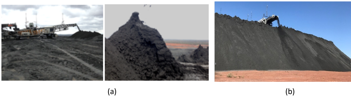
Figure 18 Effect of moisture content on stacking operation. (a) Higher than design moisture (upset conditions); (b) Design moisture content (normal condition)
