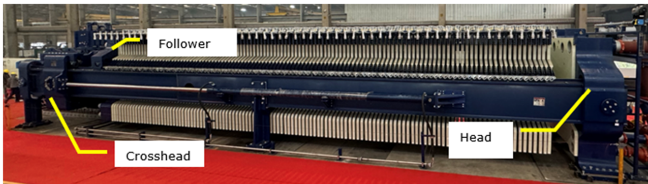
Figure 1 The major structural components of a filter press
