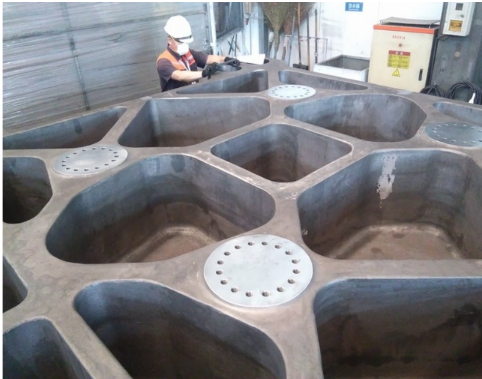
Figure 2 The AFP2500 cast follower being inspected by a quality officer
