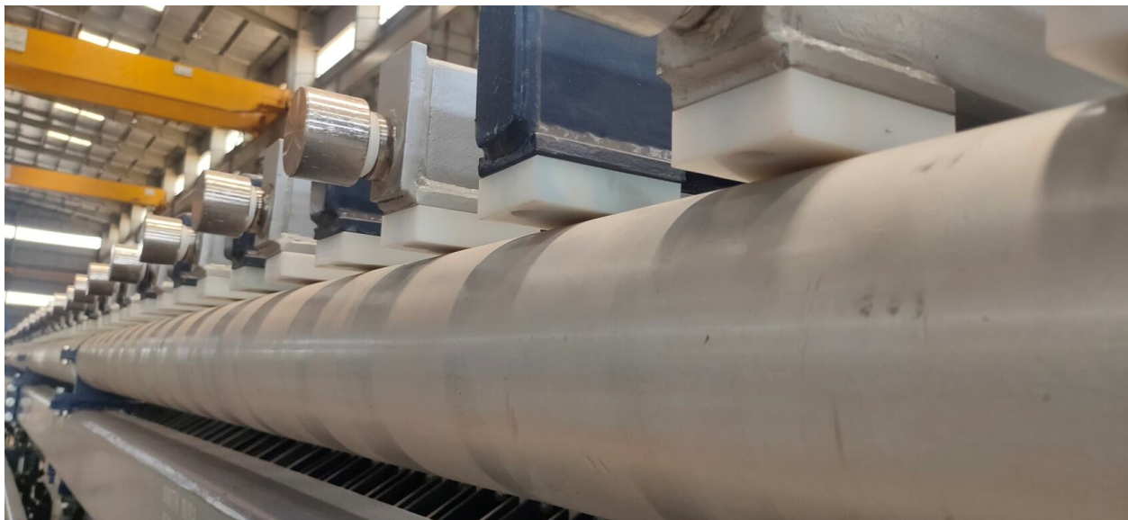
Figure 4 Photograph showing a section of the rotating elliptical pipe that forms the cloth shaker. As the pipe rotates, the shaker bars are raised and lowered
