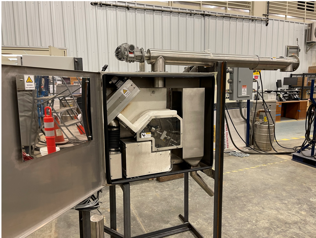
Figure 9 The first prototype Automatic Moisture Analyzer being prepared for site testing
