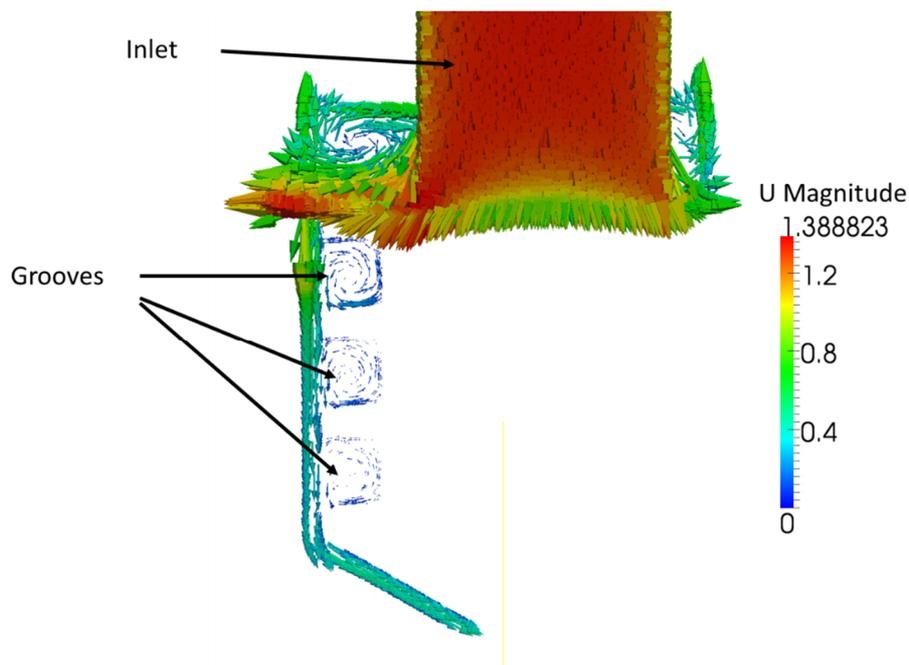
**Figure 3 Detail of flow within the grooves of the drag reduction technology**
