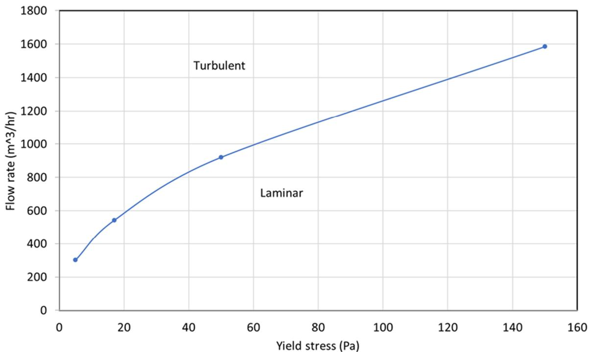
**Figure 10** Chart showing the laminar and turbulent operating regimes of the example NB 250 mm pipe system
