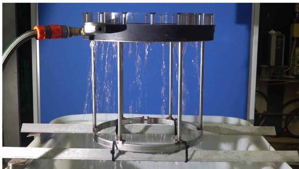
**Figure 6** Discharge from NB 250 mm drag reduction technology at  $1 \text{ m}^3 \text{ h}^{-1}$  ( $17 \text{ L min}^{-1}$ )
