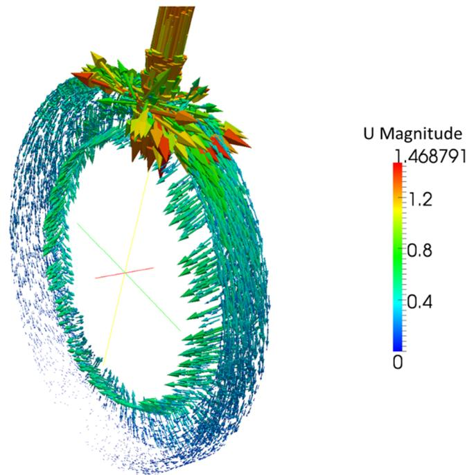
**Figure 2 Overall flow vectors throughout drag reduction technology**
