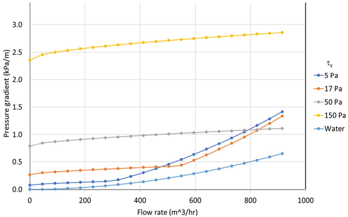
**Figure 9** Flow curves based on slurry flow rate and pressure gradient
