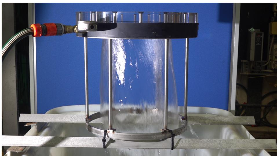
**Figure 5** Discharge from NB 250 mm drag reduction technology at  $6.8 \text{ m}^3 \text{ h}^{-1}$  ( $114 \text{ L min}^{-1}$ )
