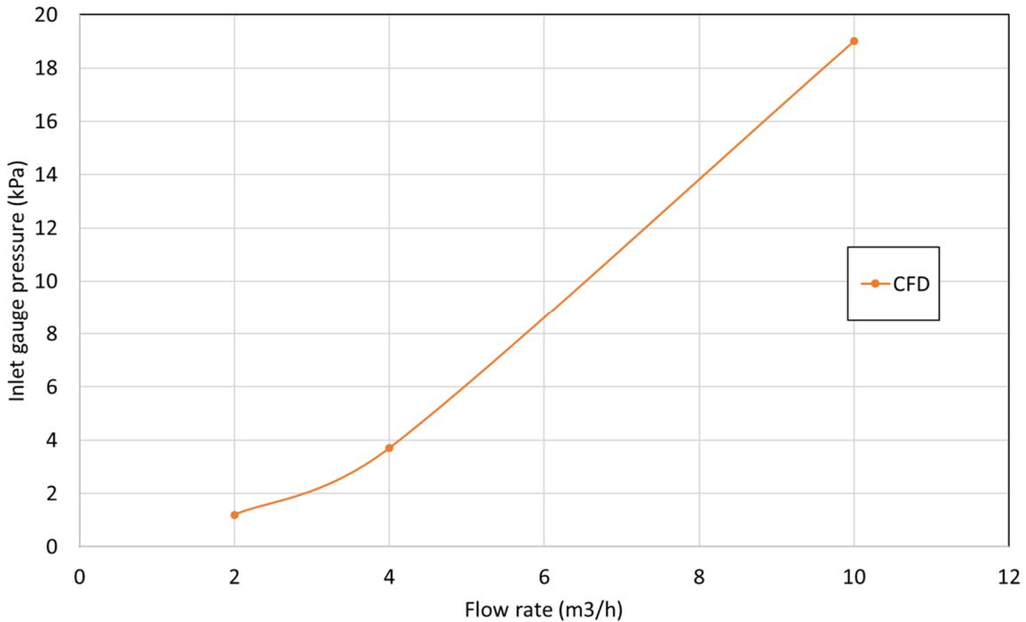
**Figure 7** Inlet gauge pressure at drag reduction technology inlet from computational fluid dynamics (CFD) runs for 250 mm NB device assuming atmospheric pressure at the outlet
