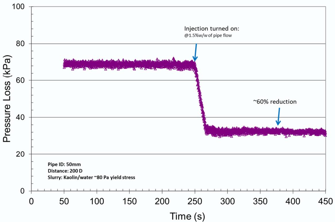
**Figure 8** Drag reduction test data from a 50 mm diameter pipe at CSIRO
