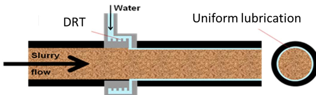
**Figure 1** Concept of CSIRO drag reduction technology (DRT)
