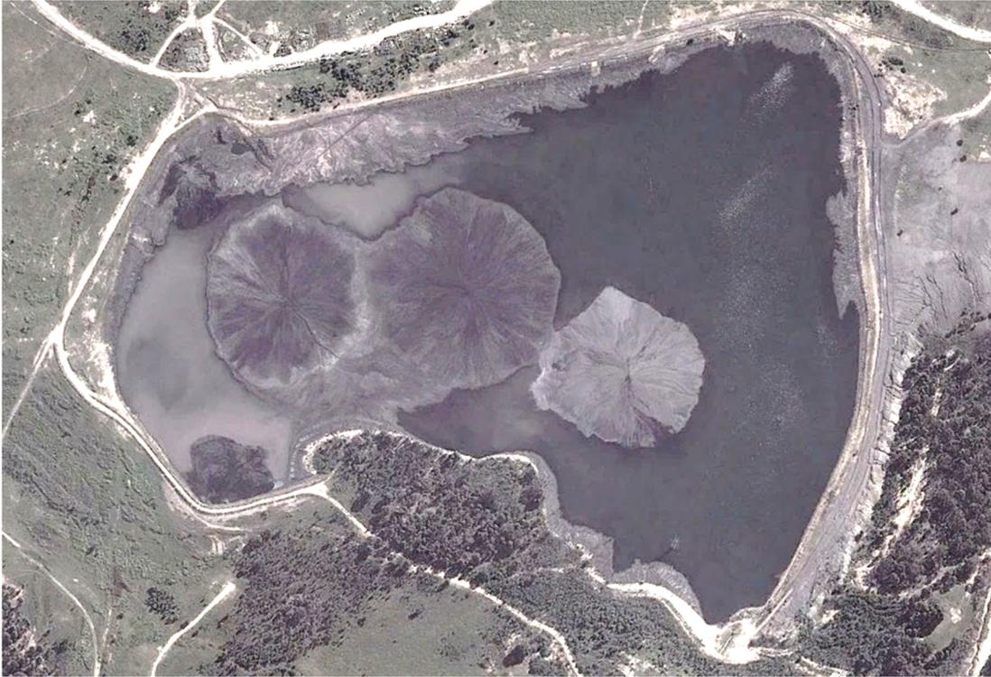
**Figure 2** Aerial photograph of Bulga's OTD dated April 2012. The three conical deposits are visible
