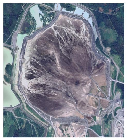
Figure 11 Aerial photograph of Musti tailings storage facility dated June 2023. The three discharge points are located at the ends of the three causeways near the south-eastern corner of the TSF
