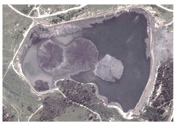
Figure 2 Aerial photograph of Bulga's OTD dated April 2012. The three conical deposits are visible
