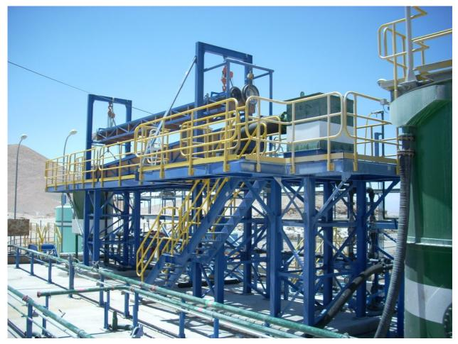
Figure 8 The 10 m long flow-through flume that was operated at Chuquicamata (Fitton 2016)
