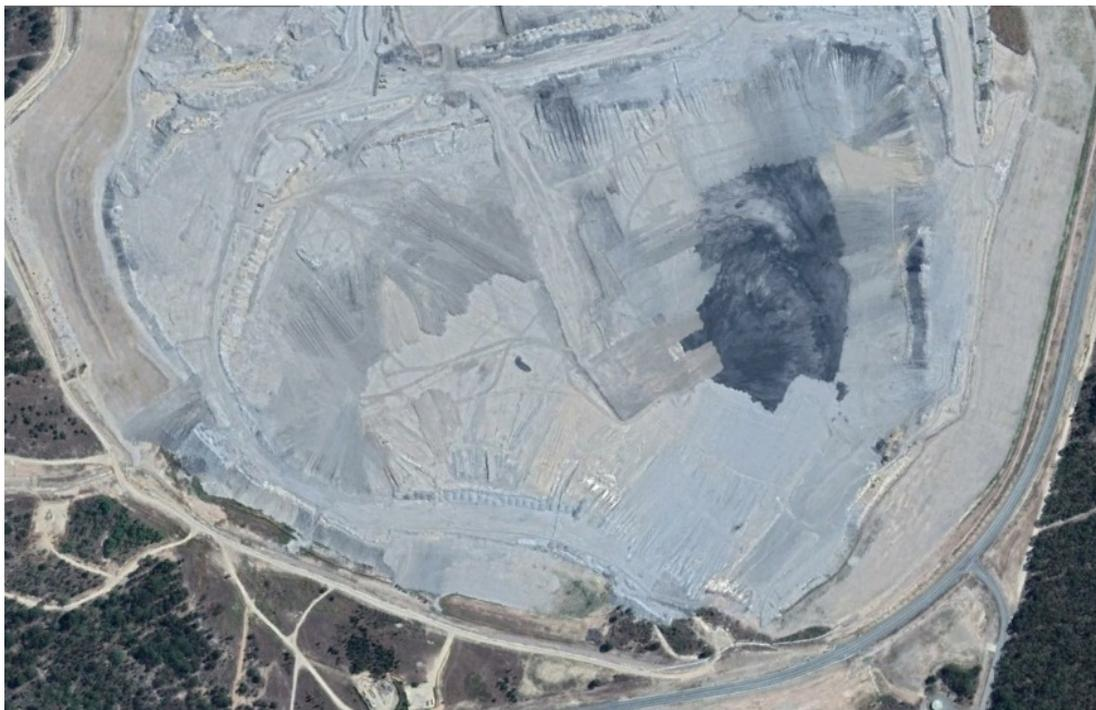
**Figure 4** Aerial photograph of Bulga's OTD dated February 2017. The capping is almost complete
