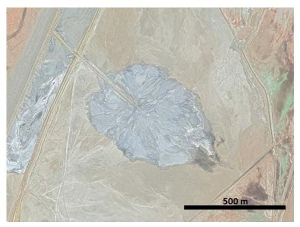
Figure 9 The trial area tailings deposit on the surface of the Talabre tailings storage facility
