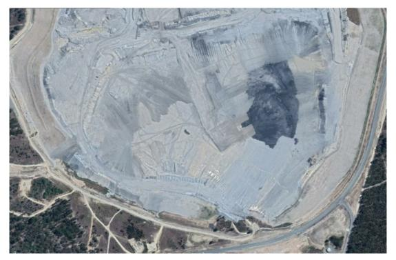
Figure 4 Aerial photograph of Bulga's OTD dated February 2017. The capping is almost complete
