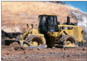
CAT 825 (Static) Tamping Foot Operating Weight – 32,750 kgs (72,200 lbs)
