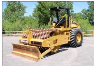
CAT 563 (Vibratory-Dynamic) Pad Foot Operating Weight – 11,570 kgs (25,500 lbs)
