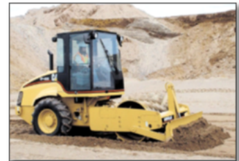
CAT 433 (Vibratory-Dynamic) Pad Foot Operating Weight – 7,170 kgs (15,800 lbs)
