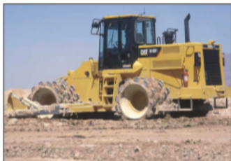
CAT 815 (Static) Tamping Foot Operating Weight – 20,770 (45,800 lbs)
