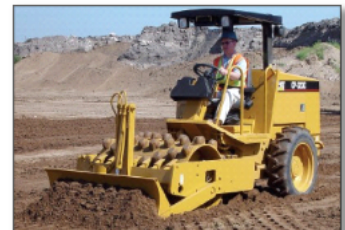
CAT 323 (Vibratory-Dynamic) Pad Foot Operating Weight – 4,630 kgs (10,200 lbs)
