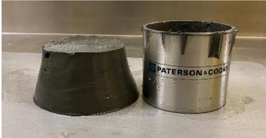
Figure 2 Photograph illustrating paste Boger slump at 76% m (2.8% binder; 280 Pa yield stress)
