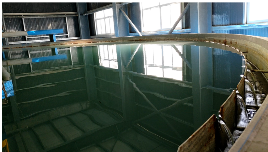
Figure 5 The overflow of the deep cone thickener
