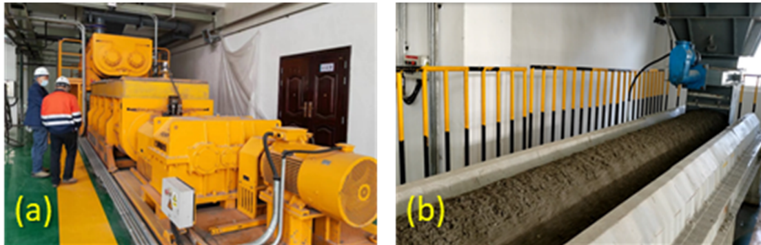
Figure 6 Mixing subsystem. (a) Two-stage double-shaft horizontal mixers; (b) Weighing belt conveyor
