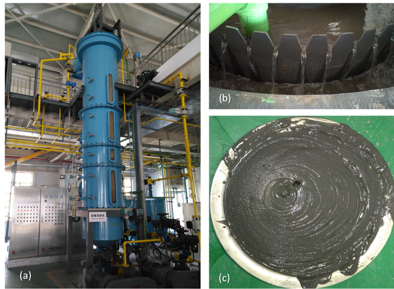
Figure 2 Flocculation and sedimentation experiment. (a) Pilot-scale deep cone thickener; (b) Overflow; (c) Underflow
