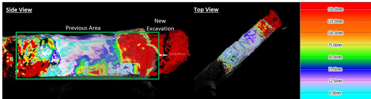
**Figure 8 Monitoring scan results during excavation measuring cumulative surface displacement**
