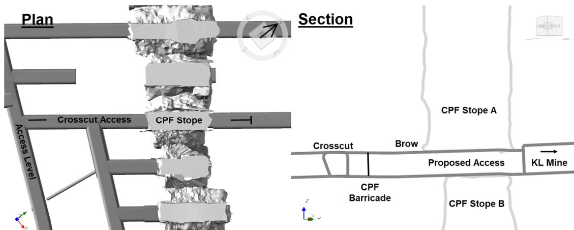
**Figure 2** Plan and section view of the proposed design cemented paste fill (CPF) drift
