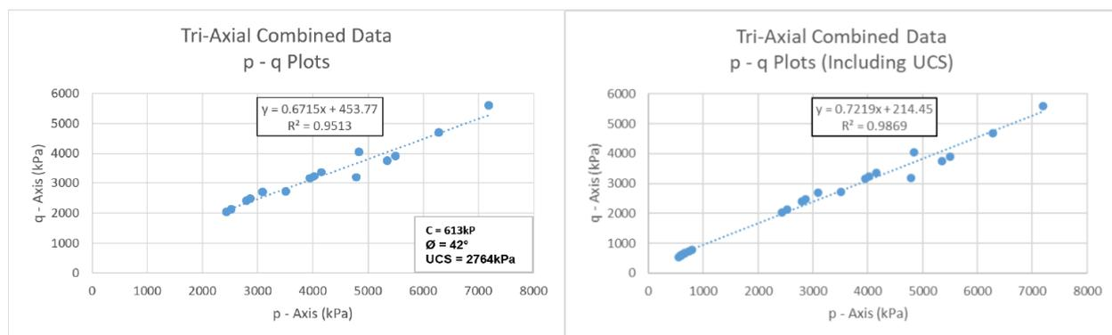
**Figure 4 Laboratory triaxial compressive strength and uniaxial compressive strength (UCS) data p-q plots summary**
