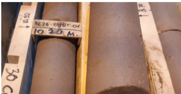
**Figure 3 Cemented paste fill core samples**
