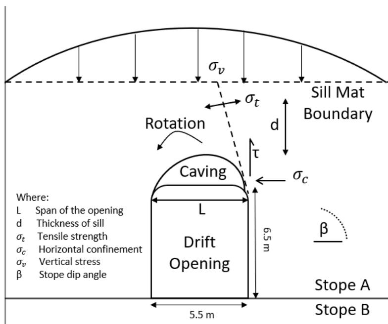
**Figure 5** Typical failure mechanisms (after Mitchell 1991)
