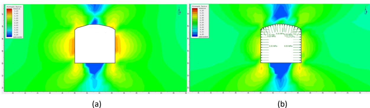
**Figure 7** (a) Strength factor of the cemented paste fill without support; (b) Strength factor with the recommended support
