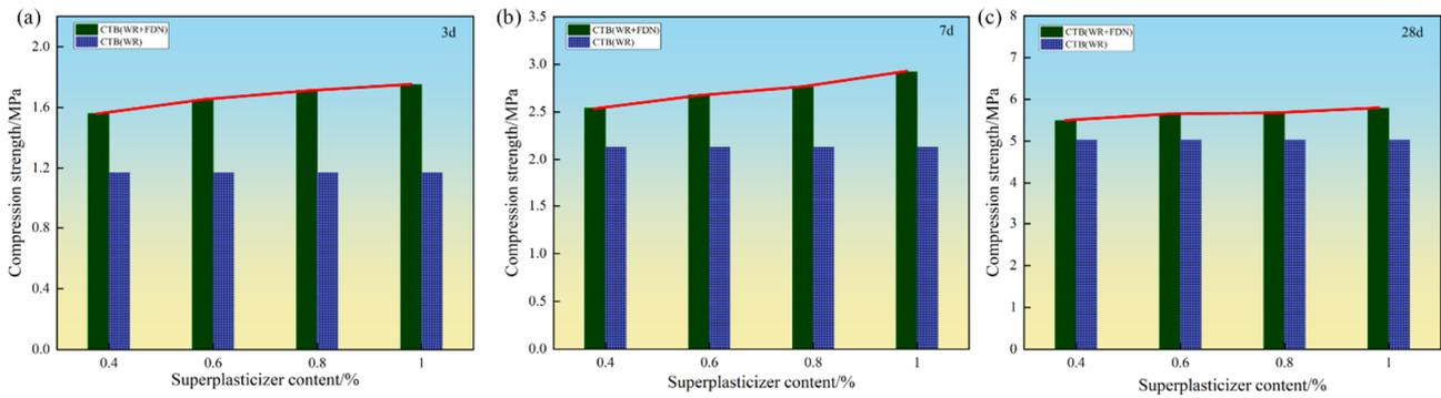
**Figure 7 Relationship between cemented paste backfill (TW+FDN) backfill strength and FDN dosage**
