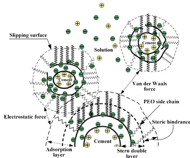
**Figure 10** The steric hindrance effects of cement particles
