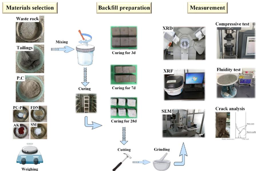
Figure 3 Experimental process and measurement methods
