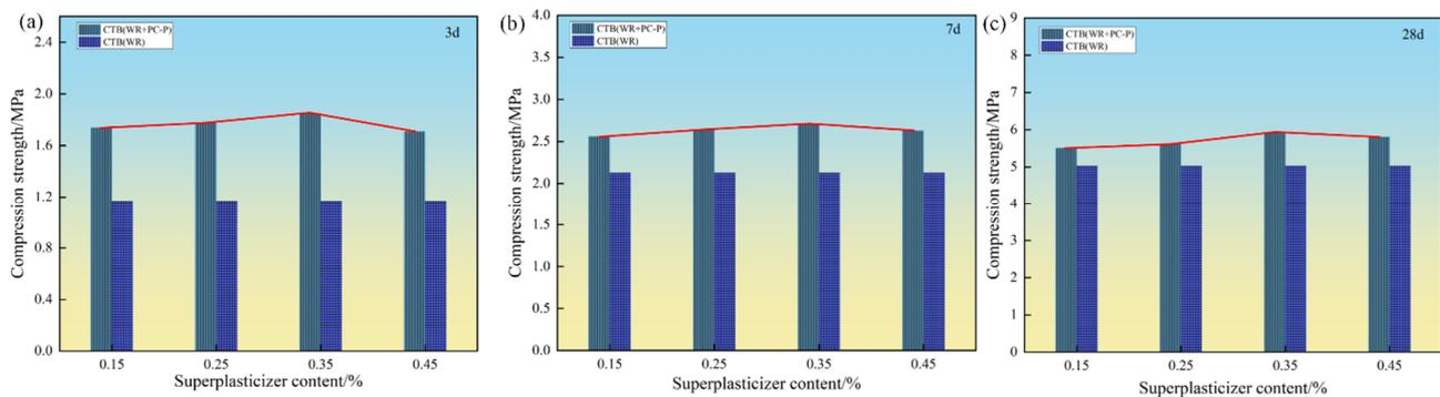
**Figure 6** Relationship between cemented paste backfill (TW+PC-P) backfill strength and PC-P dosage
