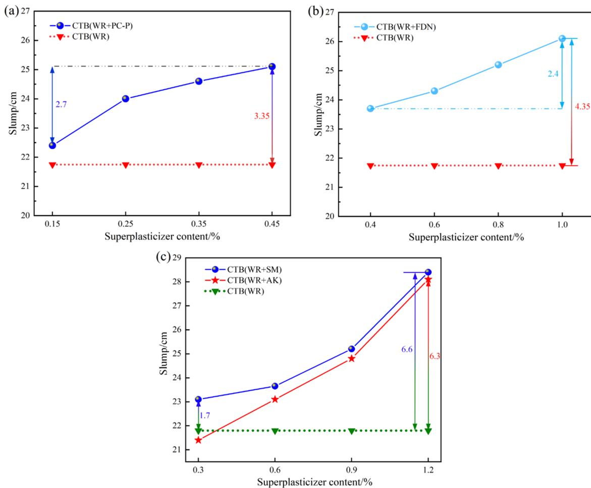
**Figure 4** Slump of CPB-TW added with different dosage of superplasticisers
