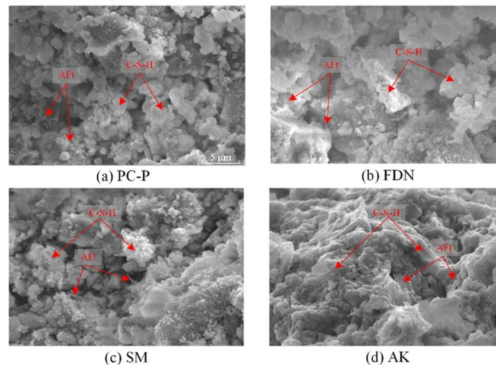
**Figure 9 Morphology and microstructure of CPB-TW hydration products**
