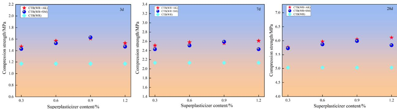
**Figure 8 Relationship between cemented paste backfill (TW+AK/SM) backfill strength and AK/SM dosage**
