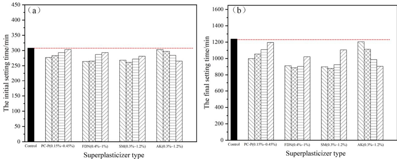
**Figure 5** (a) Initial setting time and (b) final setting time of CPB-TW with four types of superplasticisers
