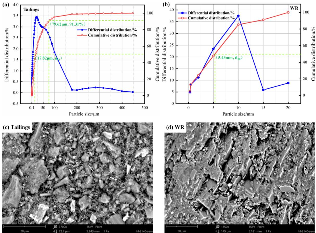
**Figure 1** Materials particle size distribution and microscopic morphology
