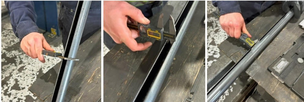
Figure 5 Examples of non-destructive geometric tests for rockbolts to verify compliance
