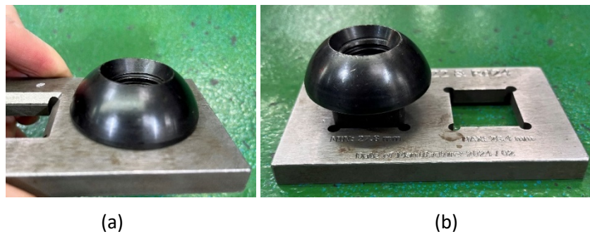
Figure 6 Examples of non-destructive geometric tests for nuts. (a) Acceptable; (b) Rejected
