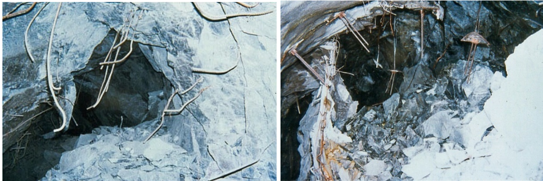
Figure 23 Examples of 'naked tendons' photographs taken by WD Ortlepp (Stacey 2016)
