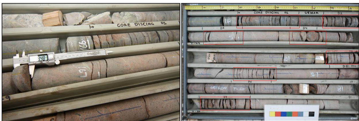
Figure 11 Core dinking in diamond core hole drilled below PC1 where a monzonite contact was intercepted. Analysis of the intervals provided the stress level for the rock
