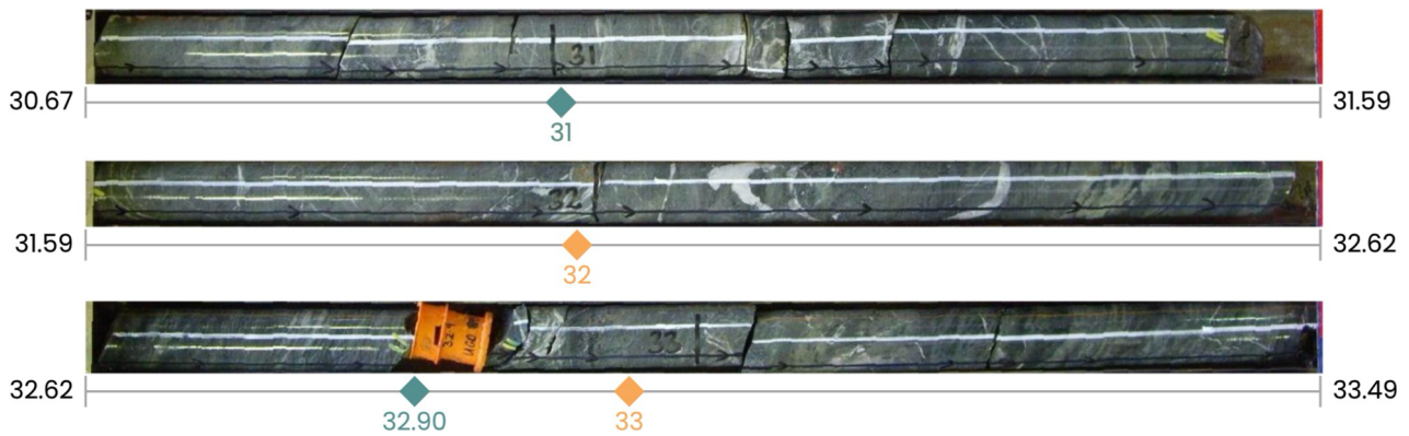
Figure 2 Example of a depth-registered core rows generated by the Datarock Core product. Each row has assigned depths from and to, including detected depths based on handwritten metre marks (green markers) and inferred depths (yellow markers)
