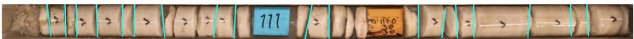
Figure 6 Example of fitted lines used to calculate the angles of fractures. The fitted lines represent the orientation of the fractures, with angles measured relative to the core axis
