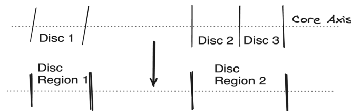
Figure 10 Example diagram showing the merging of angle-based and region-based discs into a single granular discing region-based on depth differences
