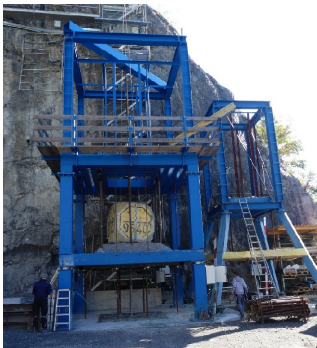
Figure 11 Walenstadt test set-up with high-tensile chain-link mesh, before lifting the test block
