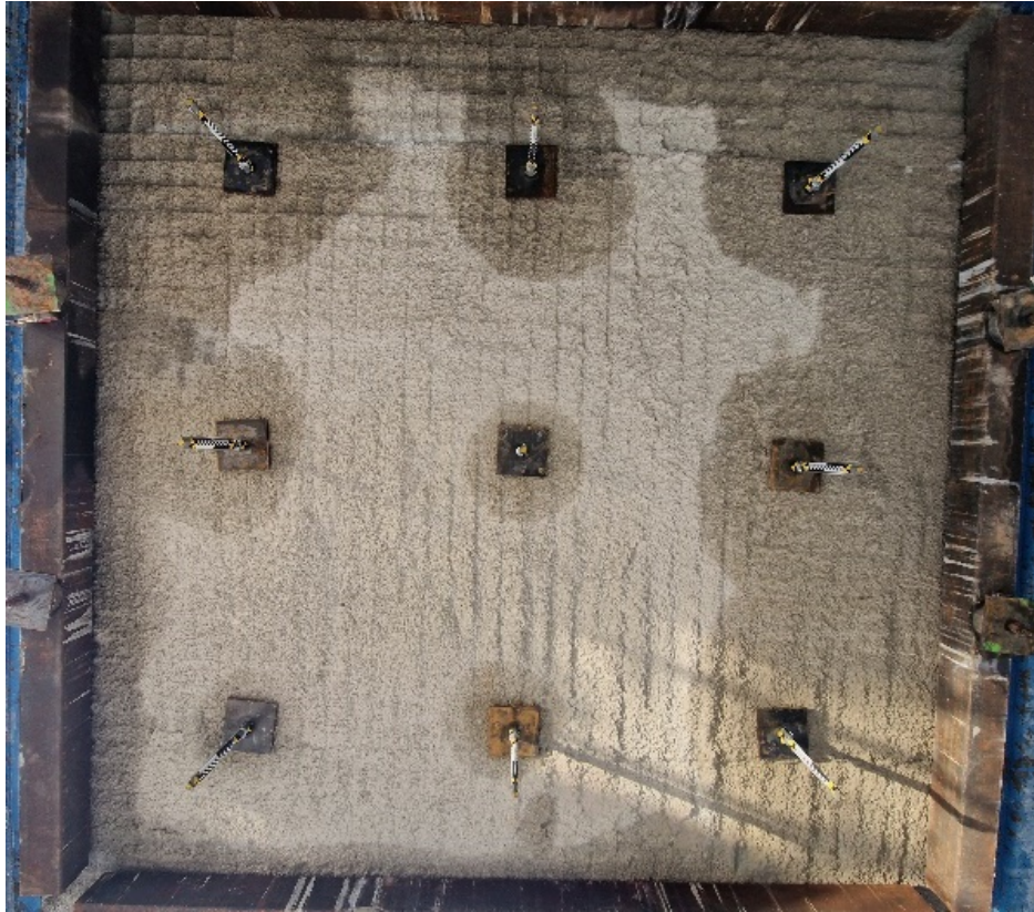
Figure 8 Configuration of welded wire mesh test
