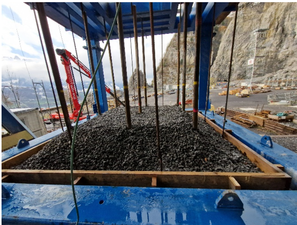
Figure 9 Simulated rock mass with 600 mm cemented aggregate fill
