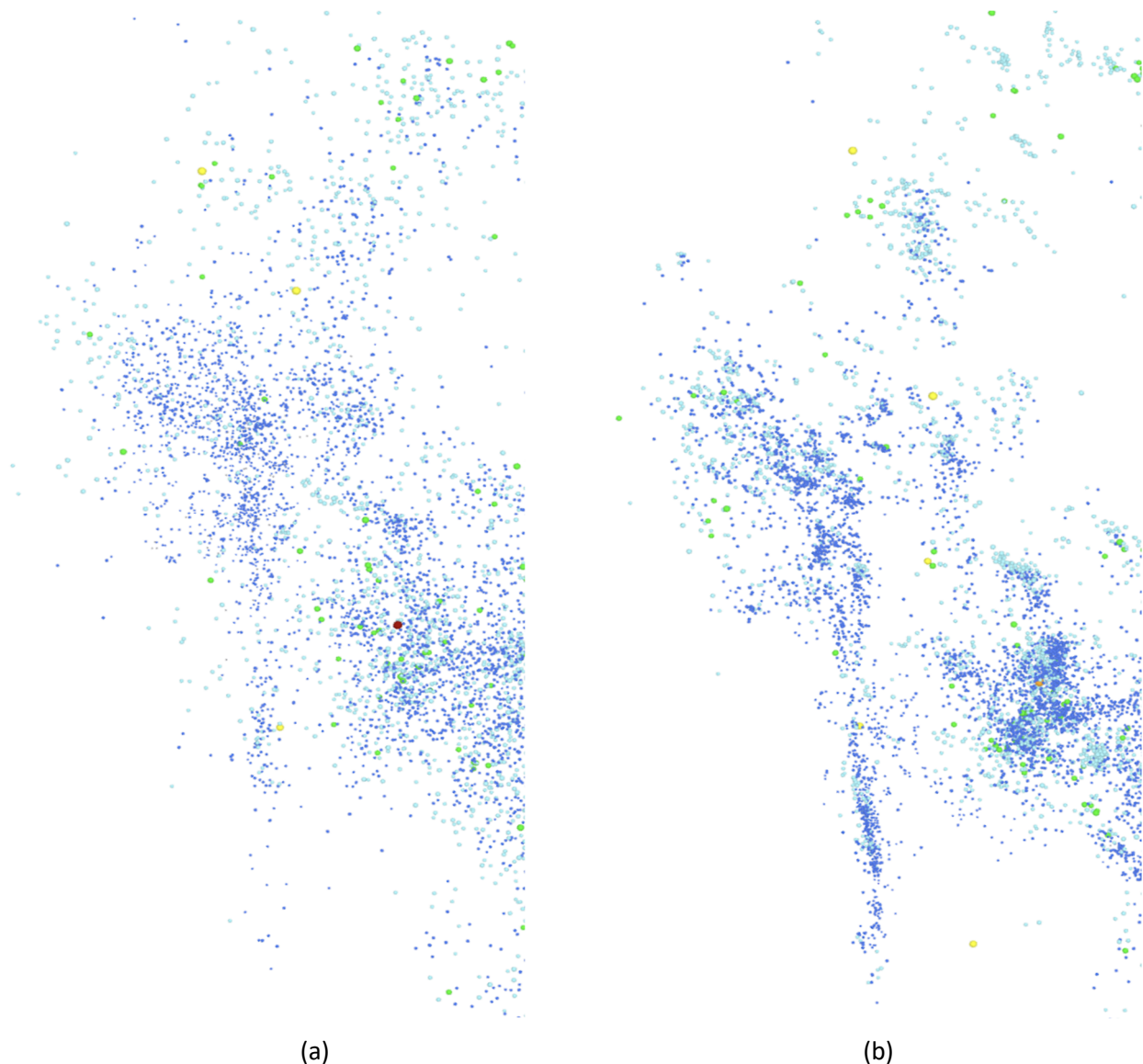
Figure 4 Comparison of self-calibration to legacy processing. (a) Shows point estimate of hypocentres of legacy processing; (b) Shows the hypocentre of accepted events estimated using BEMIS 2.0 processing after four iterations of self-calibration. Both figures are coloured by magnitude from grey to red (using the colour scale shown in Figure 7). In (b) the events are filtered with a 17 m location uncertainty to obtain a similar number of events as in the legacy processing in (a)
