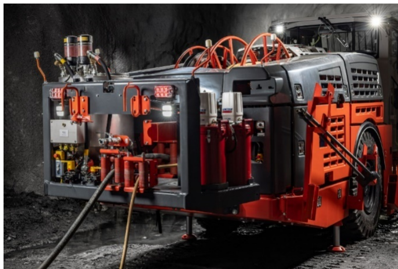
Figure 7 Sandvik DD422i-DC face drilling jumbo equipped with urea-silicate resin pumping kit
