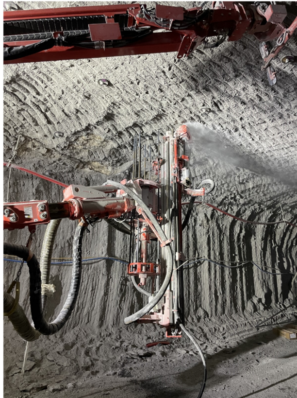
Figure 10 Sandvik DS3111 mechanised bolter drilling in the roof of the gallery. Then shooting FASLOC SF capsules for roof bolting trials (the same gallery as for SEPT tests)
