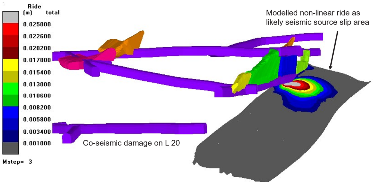
Figure 8 The same view as Figure 7, showing the third model step when the displacement-discontinuity element surface was allowed to yield in shear deformation. The outlined area simulates seismic fault slip area, which can be quantified in terms of modelled seismic potency
