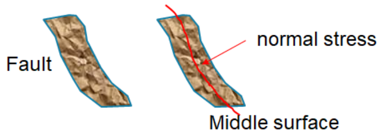
Figure 1 The middle surface obtained from the given volumetric geometry of the fault
