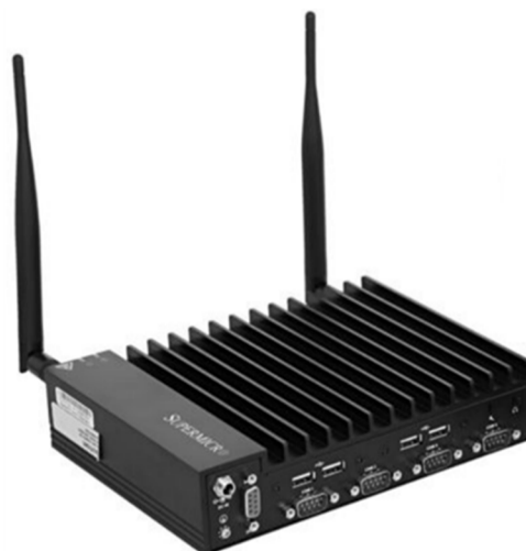
Figure 5 Supermicro server which communicates wirelessly with the tags and anchors of the ultra-wideband location system
