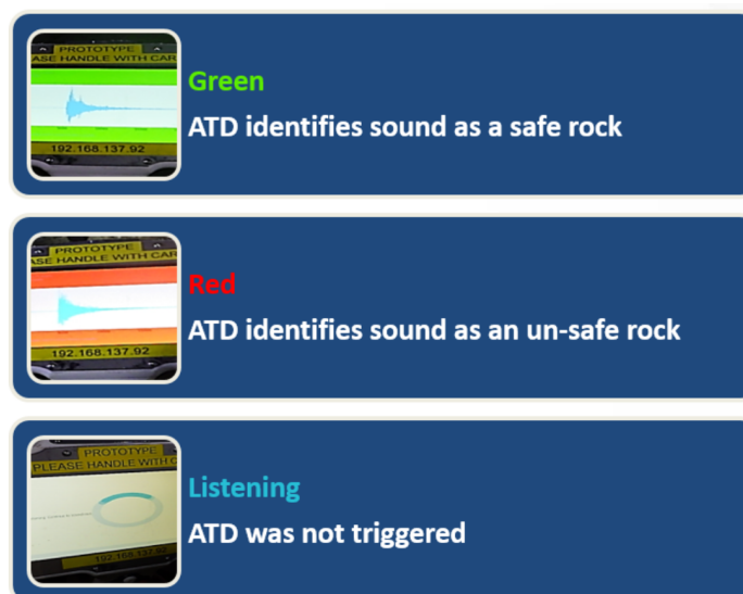
Figure 3 Acoustic thermal device read-outs delivered three results
