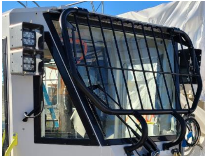
Figure 8 Equipment improvements – reinforced cabinet by bulletproof glass; rock-deferred steel screen
