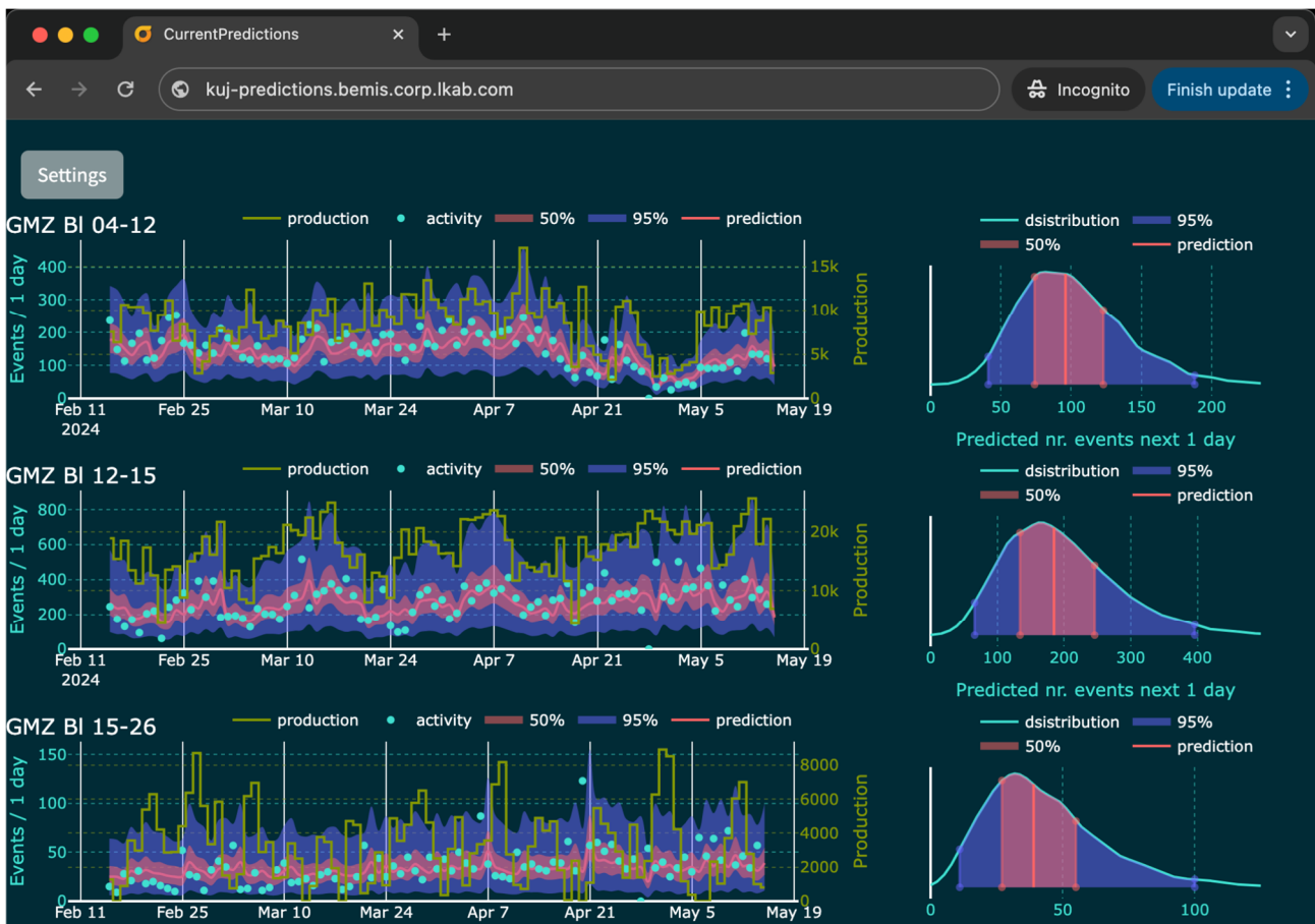
Figure 3 Daily forecasts. Visualising seismic activity, production, and activity forecasts in the first three (out of seven) volumes in the Kiruna mine. See Figure 2 for a detailed explanation of the elements of the graphs
