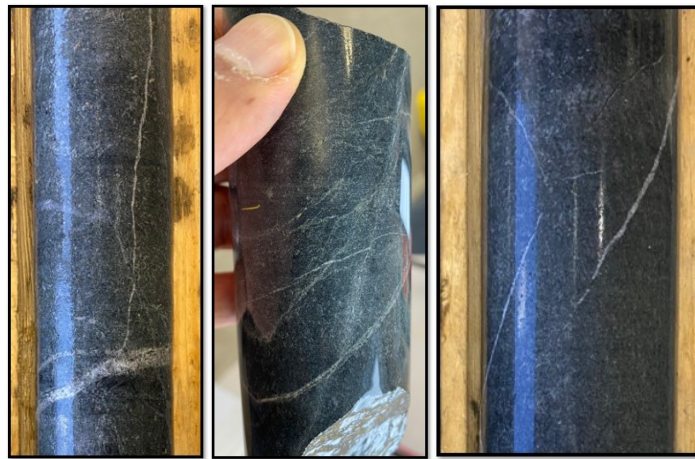
Figure 4 Natural fractures in metagabbro that are well healed with quartz infill
