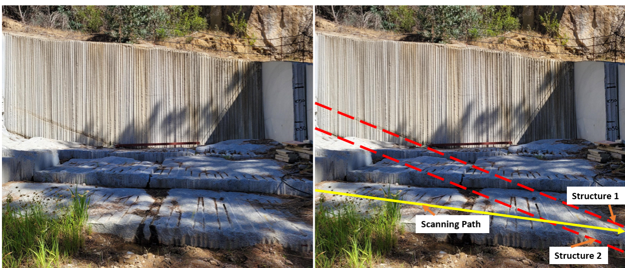
Figure 4 Granite bench with identifiable geological structures used in a baseline scan to investigate the impact of mesh aperture size
