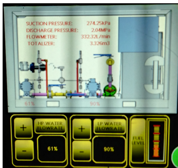
Figure 6 Operator's pump control screen
