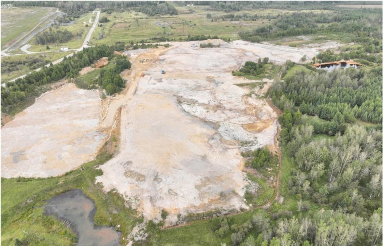
Figure 4 Industrial Area, August 2023, after the relocation of waste rock and concrete rubble to the pit
