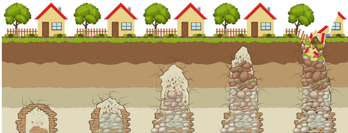
Figure 1 Formation of a localised collapse through the upward progression mechanism of a sinkhole cavity
