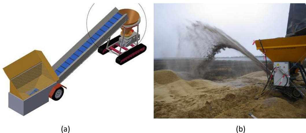
Figure 7 (a) Throwing belt principle (GMB GmbH & LMBV mbH 2025); (b) Throwing belt in test operation (GMB GmbH & LMBV mbH 2025)
