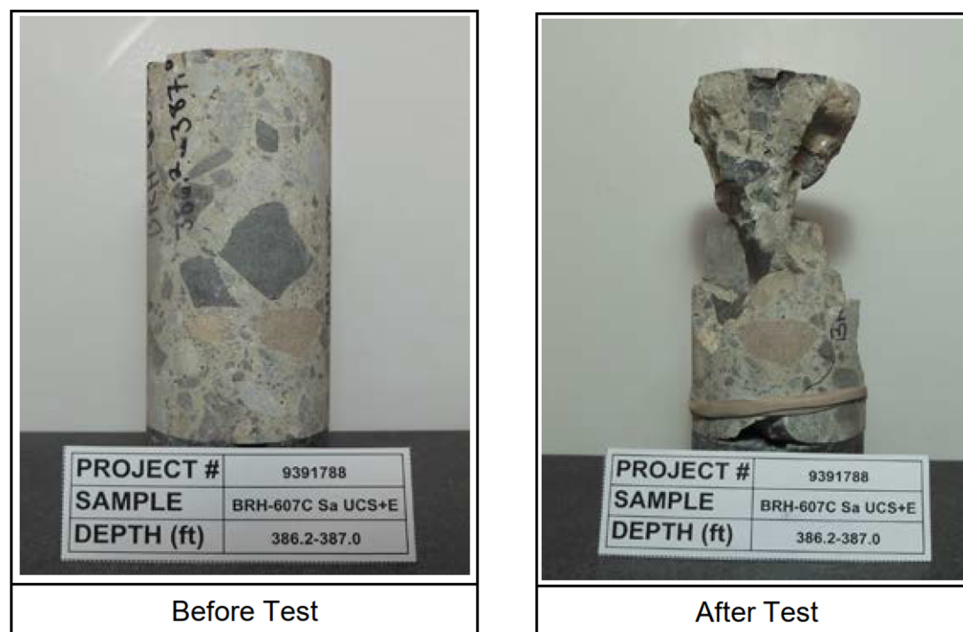
Figure 5 Strongly cemented alluvium core sample from the south wall of the East Archimedes pit
