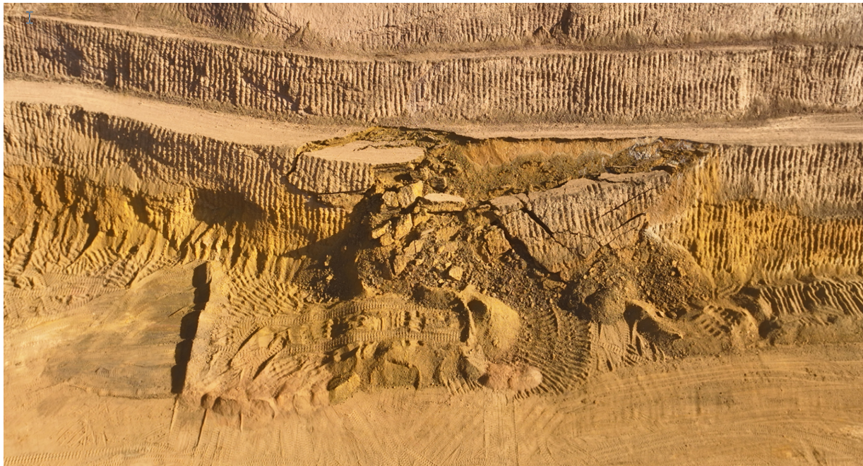
Figure 4 Unmanned aerial vehicle photogrammetry of latest Pit A slope instability post incident
