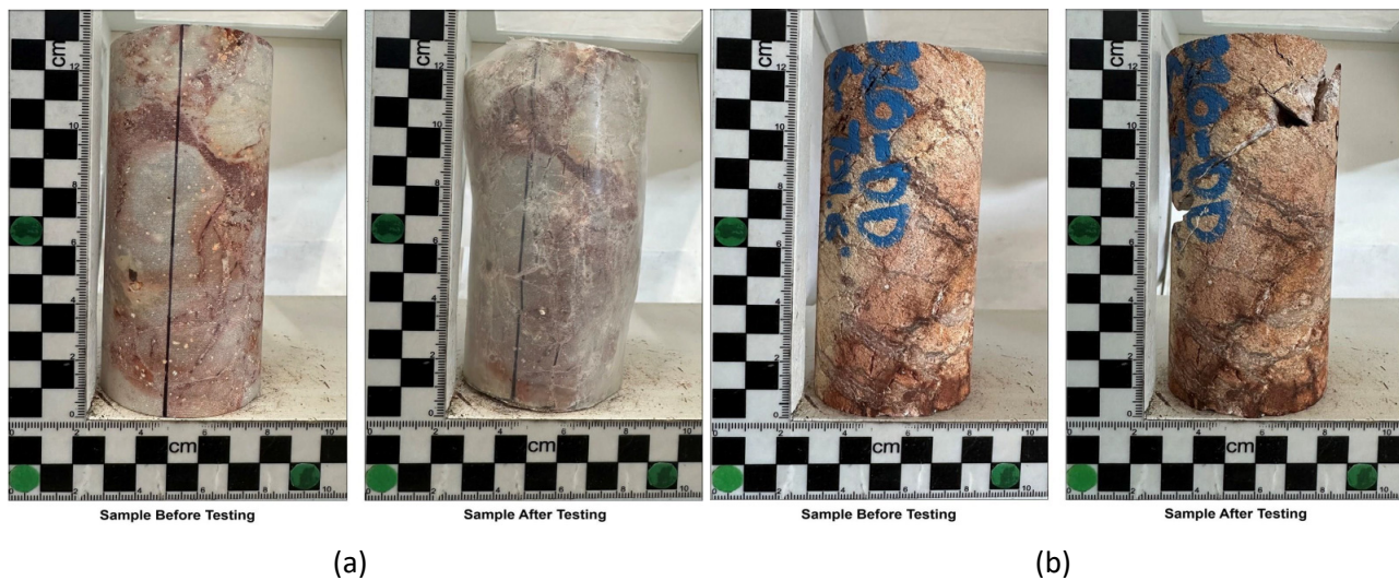
Figure 12 Typical sample failure modes axial splitting, and in shear for (a) a silica altered sample and (b) a clay altered sample
