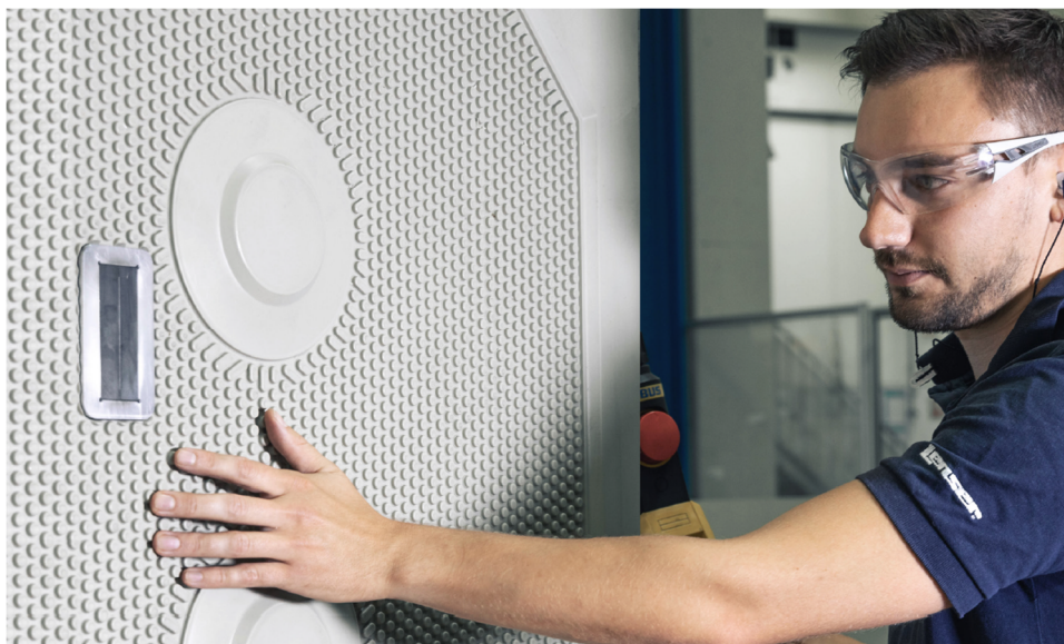
Figure 3 Plate-integrated cake water content sensor (LENSER Filtration 2024)
