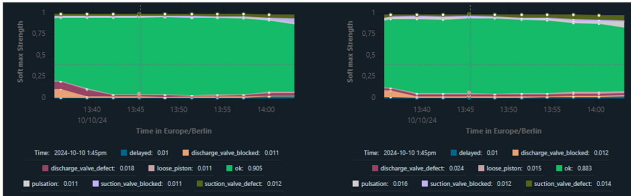
Figure 8 Positive displacement pump in good operation classified by artificial intelligence model
