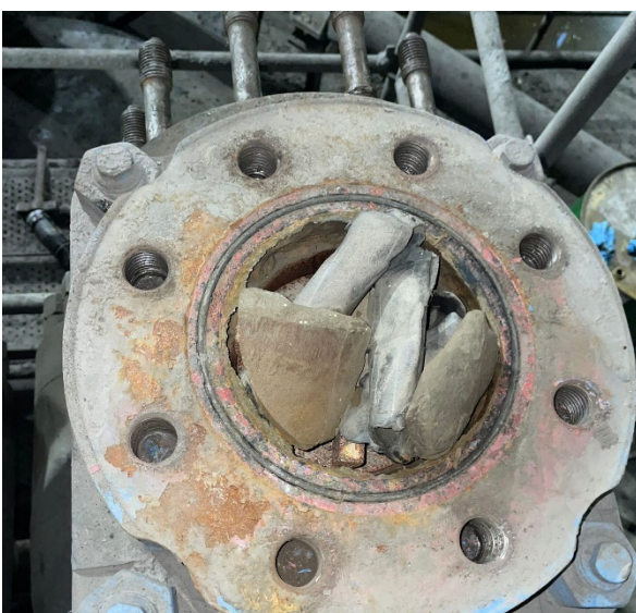
Figure 9 Positive displacement pump operation with suction valve blockage classified by artificial intelligence model
