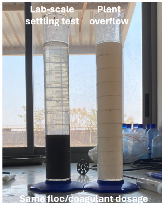
Figure 4 Laboratory simulation (left cylinder) versus overflow from the operating thickener (right cylinder) using the same reagent dosages
