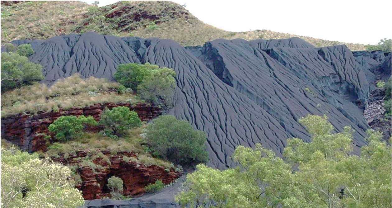
Figure 3 Unrehabilitated asbestos tailings at Wittenoom (photo credit Maurice Blackburn)
