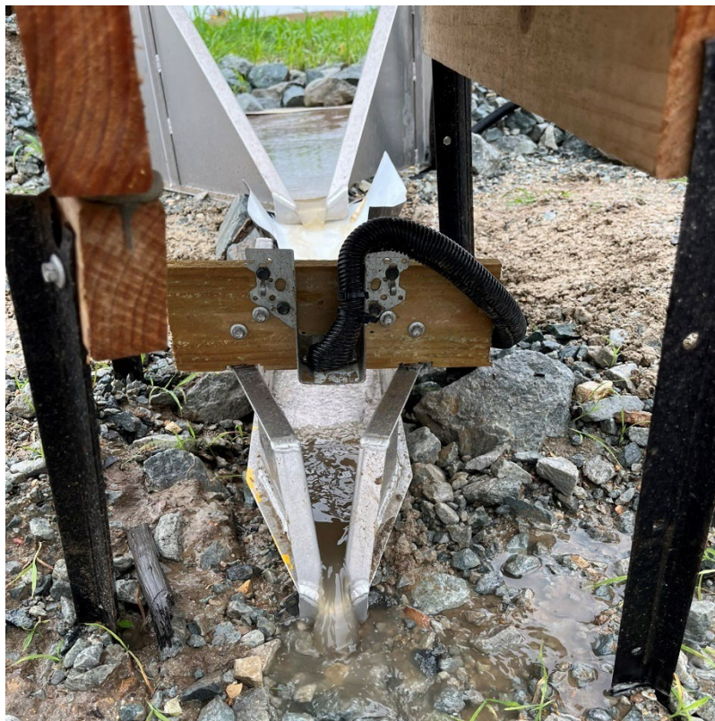
Figure 8 Flume outflow monitoring run-off
