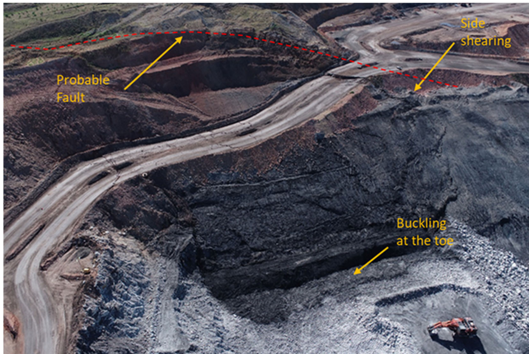
Figure 4 Unmanned aerial vehicle drone image of the initial slope movement
