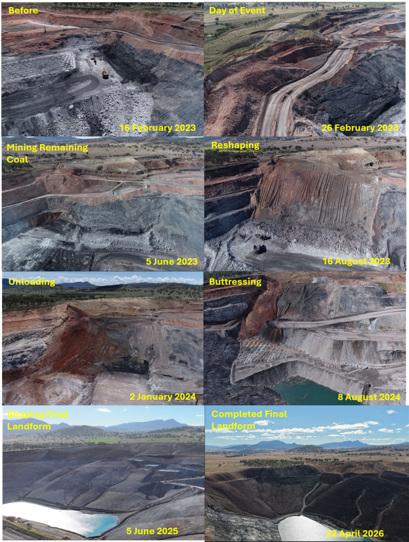
Figure 10 Eastern slope progression to final landform
