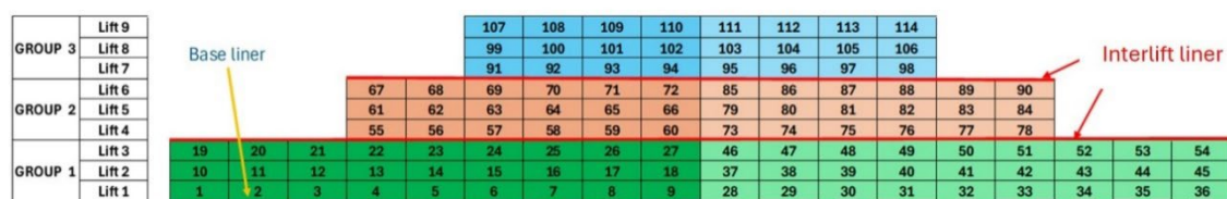
Figure 1 Schematic representation of the proposed heap leach facility geometry
