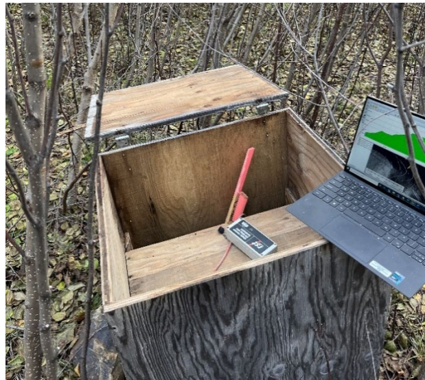
Figure 1 Plywood box constructed to protect a vibrating wire piezometer and its datalogger, its location marked with flagging tape and the shelf keeping the datalogger elevated and dry. The photo is taken 15 years after installation
