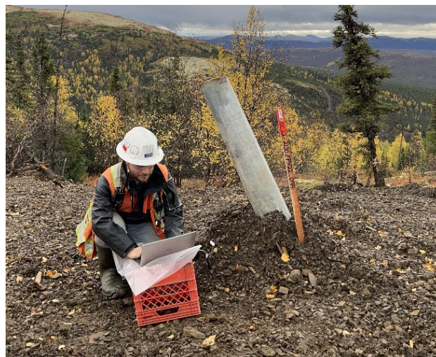
Figure 2 Collecting readings at a vibrating wire piezometer protected with a piece of culvert and capped with a rubber dock cap. This project in Alaska repurposed this leftover material from road improvements to make robust, cost-effective instrument protection
