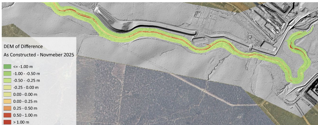
Figure 4 Digital elevation model of difference for the recently constructed diversion, exhibiting erosion and deposition as expected within the design paradigm for an alluvial low-flow channel
